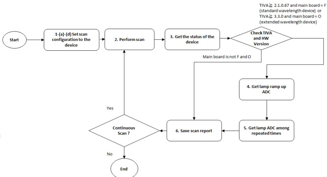
1. Set the scan configuration to the device. **(Note: This only set the configuration to the device memory and generating the scan patterns accordingly.)**
