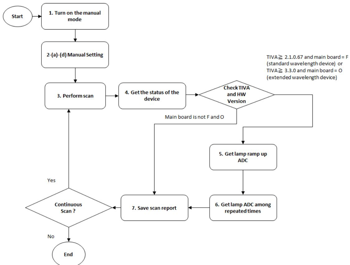
1. Turn on the manual mode will support to set lamp on or off, scan PGA and scan repeats.
