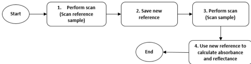
1. Place the **reference sample** and call the **PerformScan (long delaytime)** to scan the reference sample. The delay time is set to 300ms to avoid the BLE hang. In **PerformScan(long delaytime)**, call the **ISCNIRScanSDK.StartScan()** to trigger the scan event. You should register **ScanDataReadyReceiver** to get the scan result.
