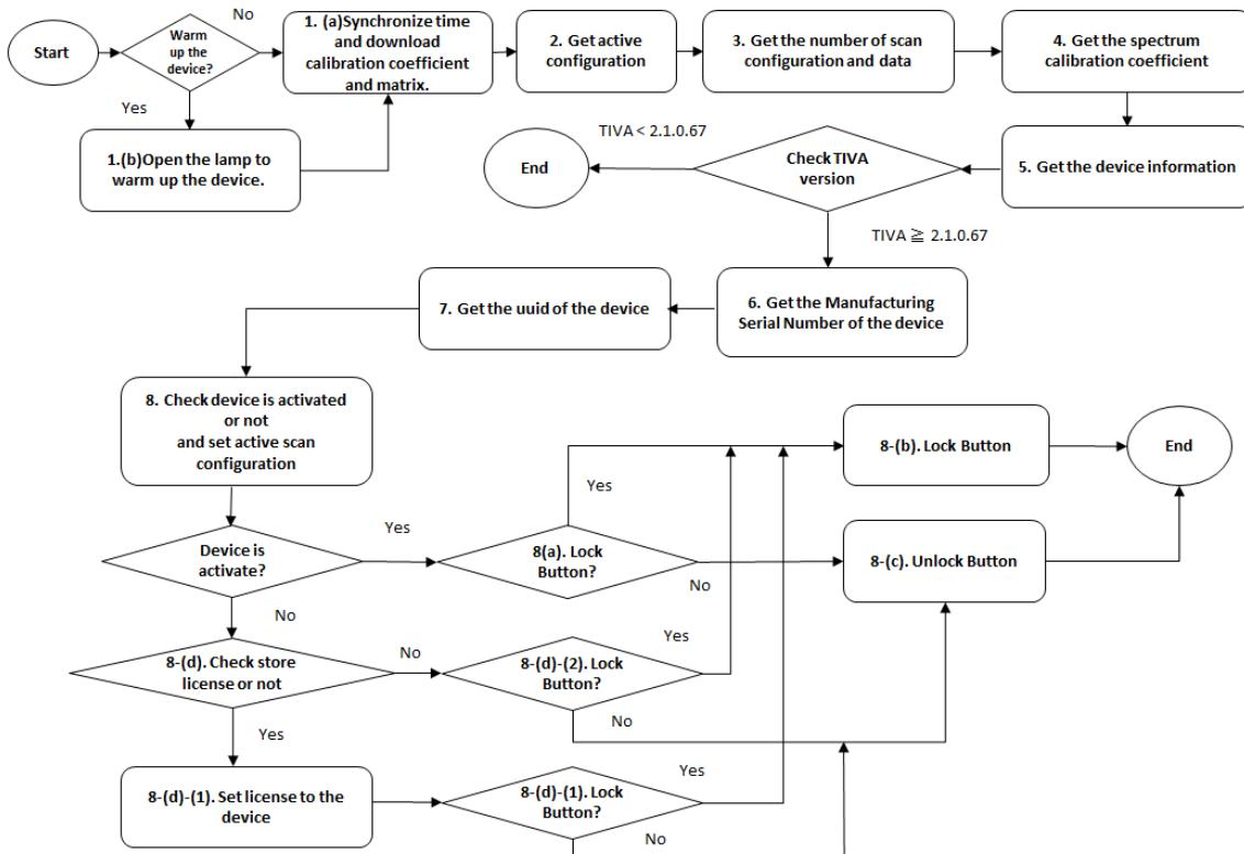
1. When the device is connected, it will first check whether the user want to warm up the device.
