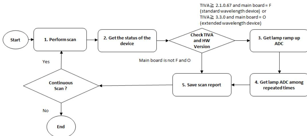
1. Call the **PerformScan(long delaytime)** to scan the sample. The delay time is set to 300ms to avoid the BLE hang. In **PerformScan(long delaytime)**, call the **ISCNIRScanSDK.StartScan()** to trigger the scan event. You should register **ScanDataReadyReceiver** to get the scan result.
